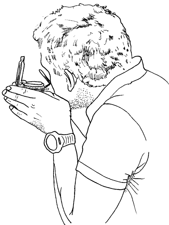
Sighting with a Lensatic compass
