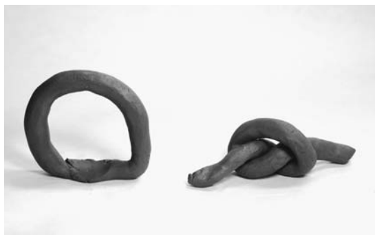
Clay field-quality test
