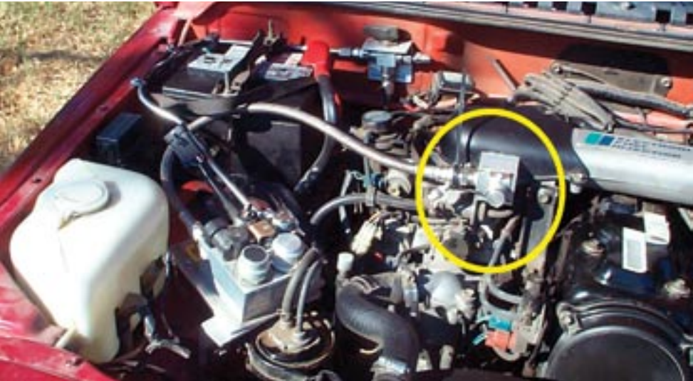
Custom machined fuel block and h2 injector
