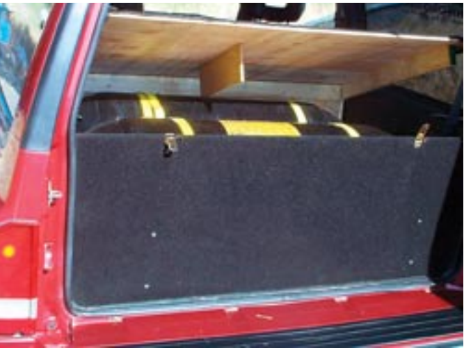
Custom built box to enclose the tanks
