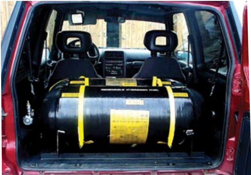
Two 61 liter 3600 psi fuel tanks with temporary mounting
