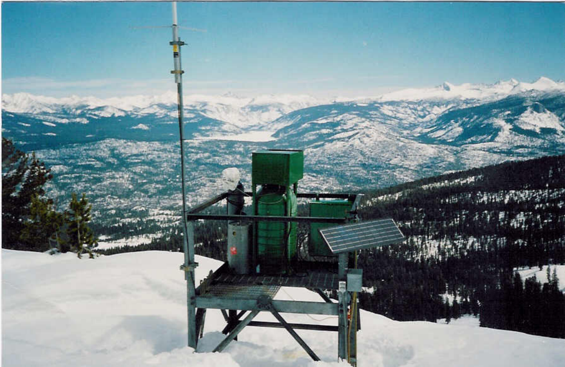
Figure 3.3 Remotely Controlled, Ground-based Silver Iodide Generator
