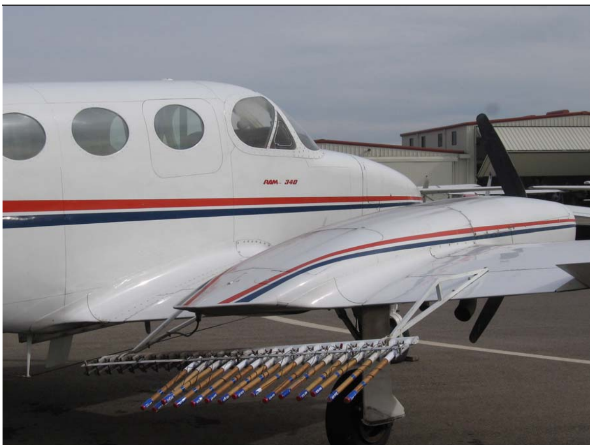
Figure 3.6 Aircraft with Seeding Flare Racks
