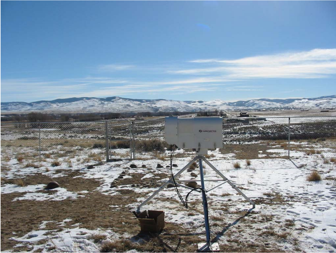
Figure 8.2 Example of a Portable Microwave Radiometer
